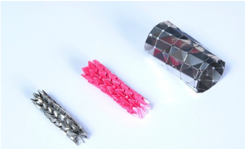
Figure 7: deployable origami stent, made from shape memory alloy [9].
